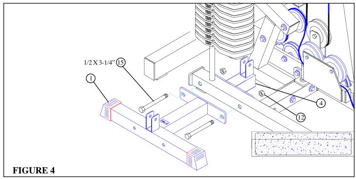
Securely fasten the FRONT LEG (1) and the BASE CONNECTION (4) to the 440 HOME GYM using two 1/2 X 3-1/4" BOLTS ٠ (15) and two 1/2" LOCKNUTS (12). See FIGURE 4.
